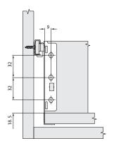
( ) Inner Drawer \*Add 8mm when used with 201.000 Drawer Front Locking Piece.
